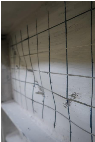
Fig. 2: Subpanel buckling during experiment [27]
