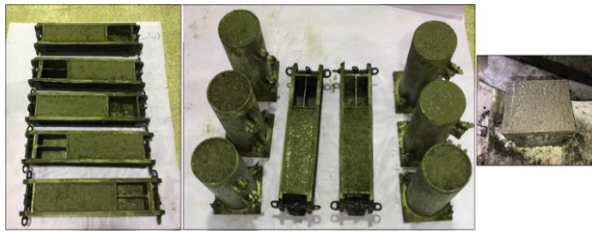
Fig. 7: Casting of Cylindrical, Beam, and Cubic specimens
