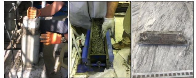
Fig. 6: Compaction of cylindrical and beam specimens using a vibration table with static load
