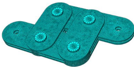
Fig. 2: Rotational friction damper
