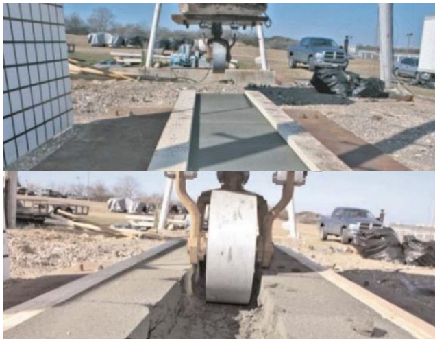
Fig. 2: Overview of pendulum test for glass foam [6].
