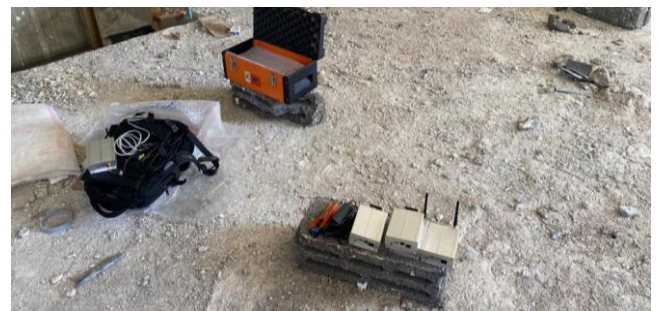
Fig. 14: Ambient vibration instruments.
