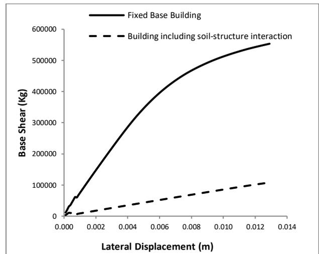
Fig. 8: Global force-deformation curve from nonlinear static analysis in the x direction.
