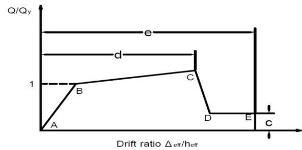
Fig. 1: Generalized force-deformation relation [13].
