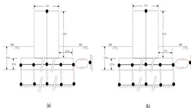
**Fig. 5:** Schematic diagram of superstructure-foundation system a) z direction, b) x direction.
