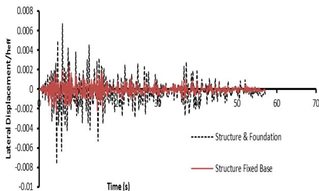
Fig. 10: Comparison of time history drift response during Qazvin\*-C3 earthquake.
