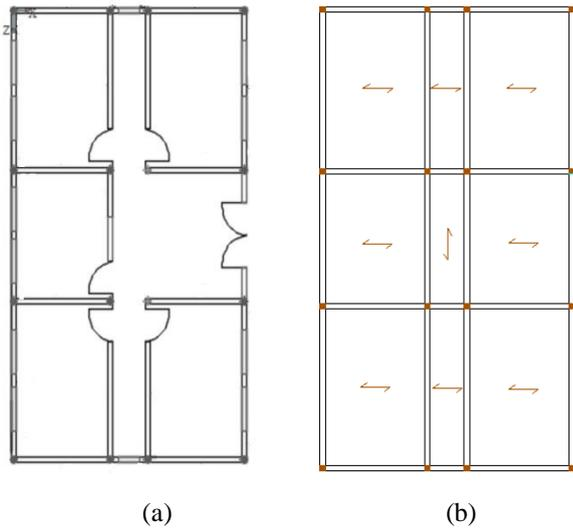
Fig.6: Building plan and its roof beam direction
