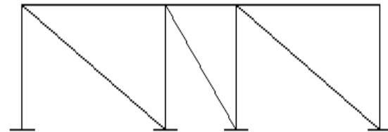
Fig. 2: Modelling of masonry walls as compression diagonal members.
