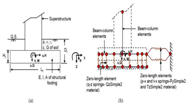
**Fig. 3:** Schematic represents diagram (a) superstructure-foundation system and (b) BNWF showing springs with their orientations [1].
