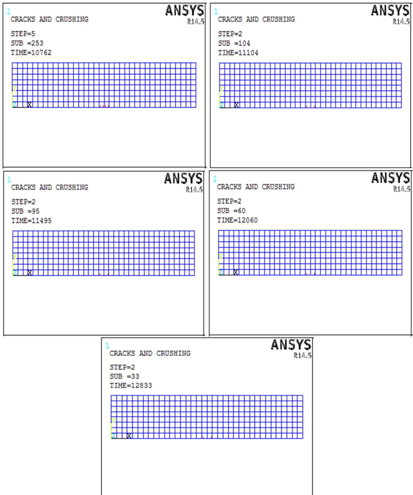
Fig. 5: First cracking of single FE model for each Beam Series
