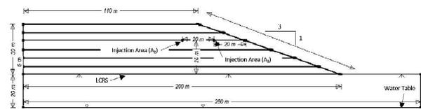
**Fig. 1:** The geometric design of conceptual bioreactor landfill.
