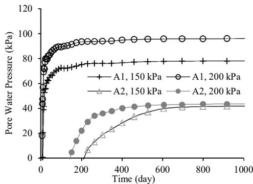
**Fig. 3:** Distribution of pore water pressure by time
