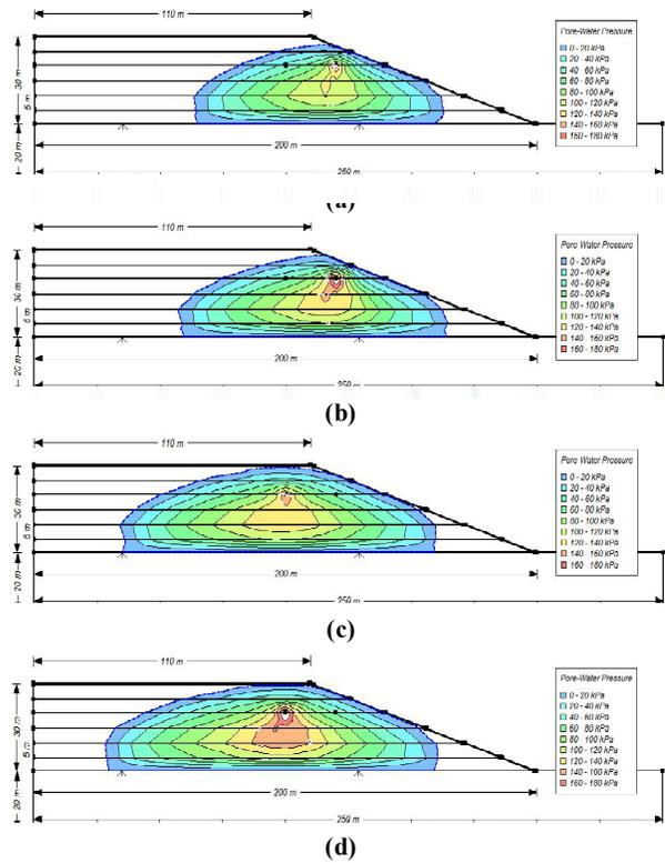
**Fig. 4:** Pore water pressure distribution under different injection pressures (a): 150 kPa for A1; (b): 200 kPa for A1; (c): 150 kPa for A2; (d) 200 kPa for A2.
