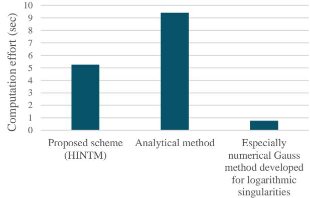
**Fig. 8:** Comparison of the computational efforts in different integration methods for solution of the heat flow example
