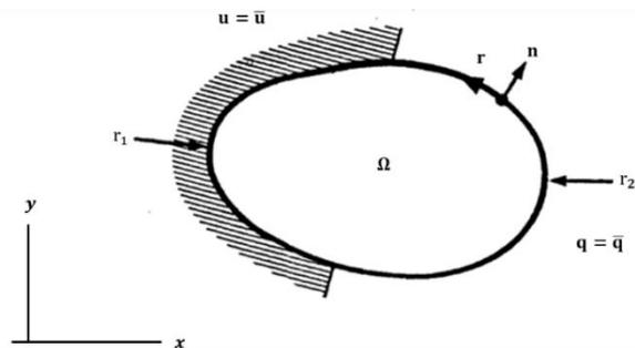
**Fig. 1:** The natural and the boundary conditions for an arbitrary Laplace problem
