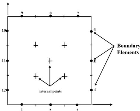
**Fig. 7:** Position of internal points and boundary elements
