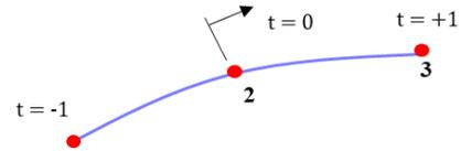
Fig. 2: Local coordinate system laid on a typical element
