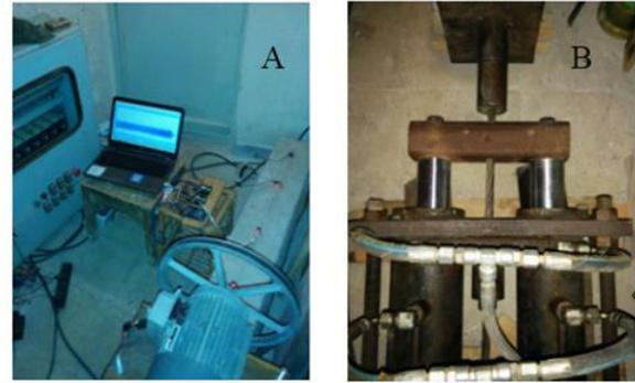
**Fig. 2:** A: View of the tests B: Prestress jack
