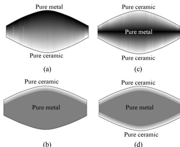
**Fig. 1:** Various types of circular plates with variable thickness: (a) one-sided FGM plate with volume fraction dependent on thickness; (b) one-sided FGM plate with a FGM layer of constant thickness; (c) bimorph FGM plate with volume fraction dependent on thickness; (d) bimorph FGM plate with a FGM layer of constant thickness
