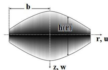
**Fig. 2:** Geometry of the circular bimorph FGM plate with variable thickness
