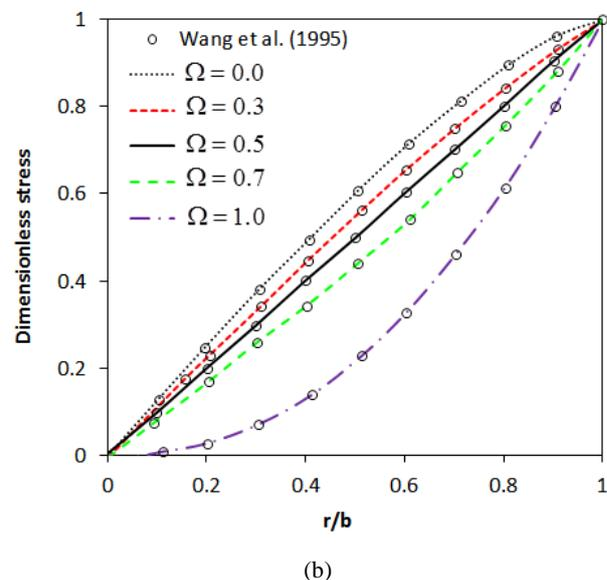
**Fig. 4:** Variations of dimensionless stress function against dimensionless radial coordinate for different values of the taper parameter  $\Omega$ : (a) linear thickness variation; (b) parabolic thickness variation
