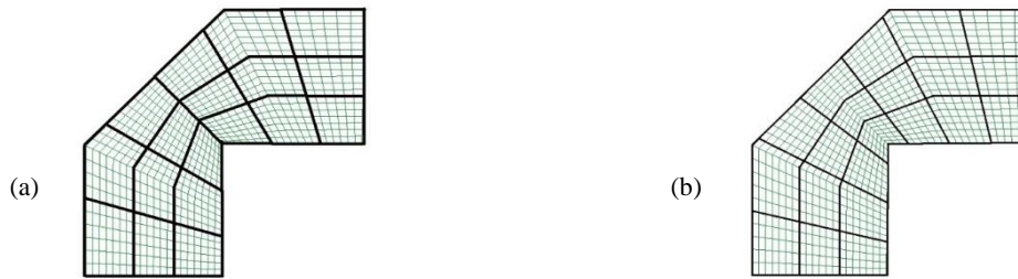
Fig. 2: Optimal substructuring of cross-shaped plate with respect to a) FLOPS cost; b) memory cost
