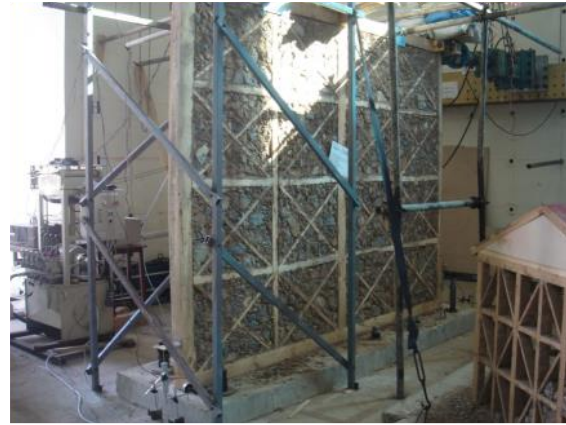
4: Experimental setup for testing of Dhajji wall
