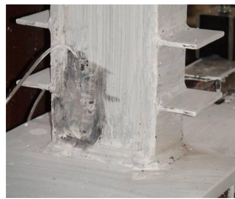
Fig. 10: The model and specimen 4 at the initial yielding: a) Equivalent plastic strain; b) Von Mises stress c) White wash splashing in the specimen
