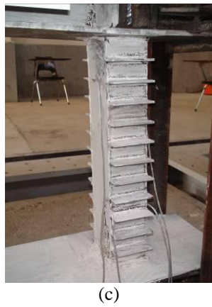
Fig. 9: The model and specimen 2 at the end of loading: a) Equivalent plastic strain; b) Von Mises stress c) White wash splashing in the specimen
