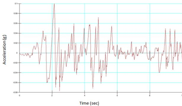
**Fig. 6:** Accelerograph used in analyses maximum acceleration  $0.1g$
