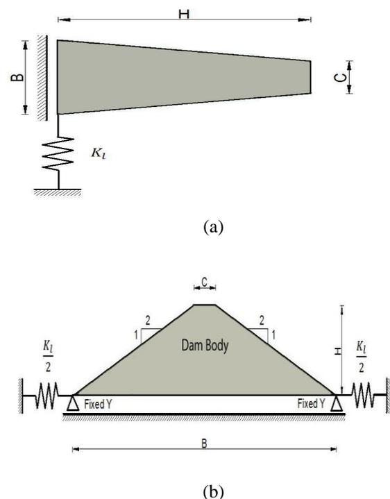
Fig.1: Generalizing the beam to earth dam
