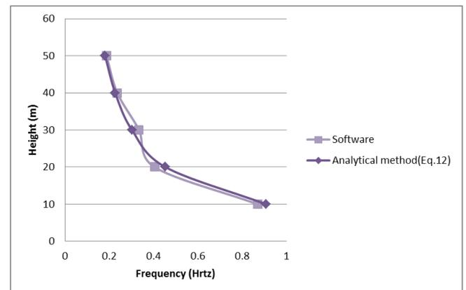
**Fig.8:** A comparison between the proposed equation and software results
