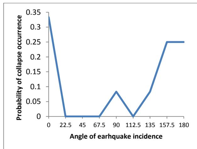
**Fig. 9:** The probability of collapse occurrence for each angle as critical
