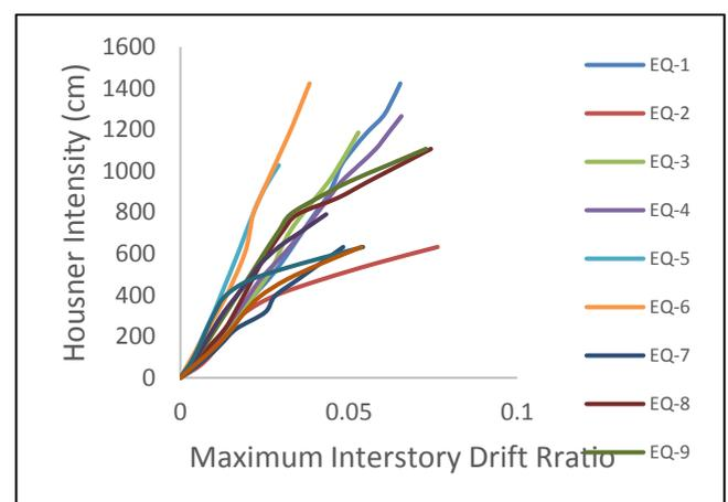
Fig. 7: diagrams of DMIDA results for maximum EDP
