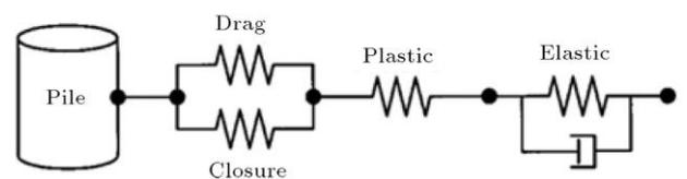
Fig. 3: Components of nonlinear p-y elements
