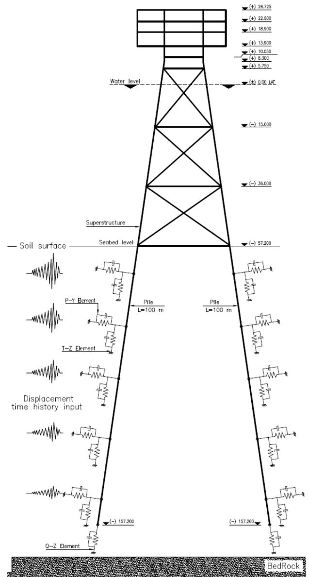
Fig. 2: Schematic view of SPD13 wellhead platform
