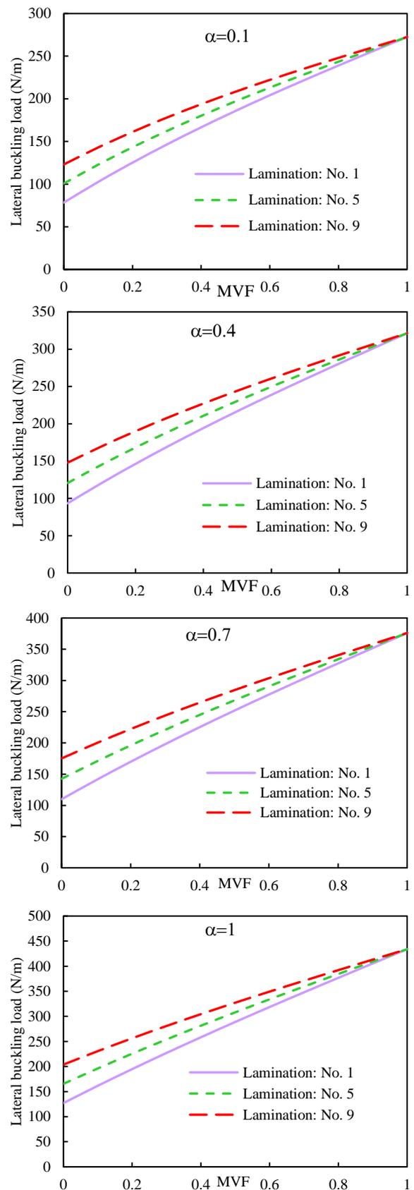
**Fig. 4:** Variation of the lateral buckling load with respect to metal volume fraction change: effect of different sequences of laminations, for different tapering ratios, and for a transverse load applied on the top flange
