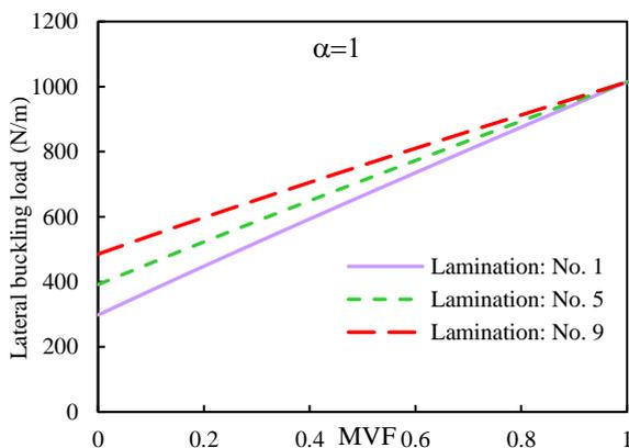
**Fig. 5:** Variation of the lateral buckling load with respect to metal volume fraction change: effect of different sequences of laminations, for different tapering ratios, and for a transverse load applied at the centroid
