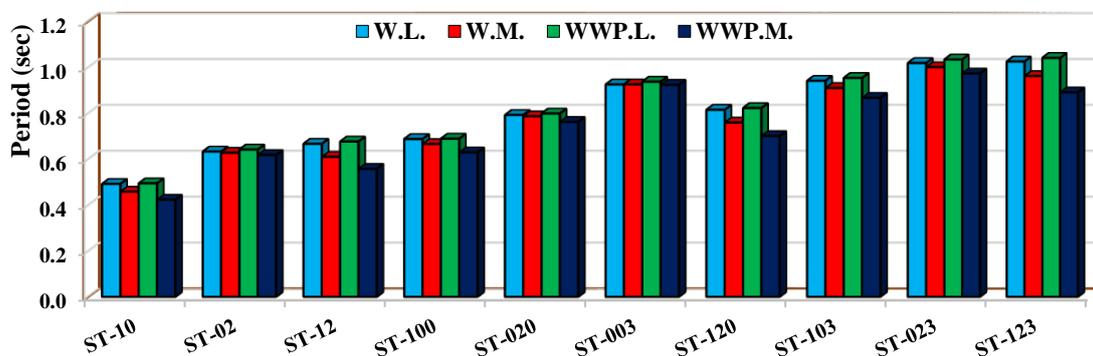
**Fig. 6:** Fundamental period in four types of analysis
