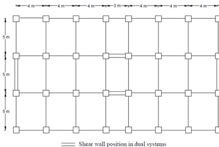
**Fig. 2:** the plan of modeled RC buildings
