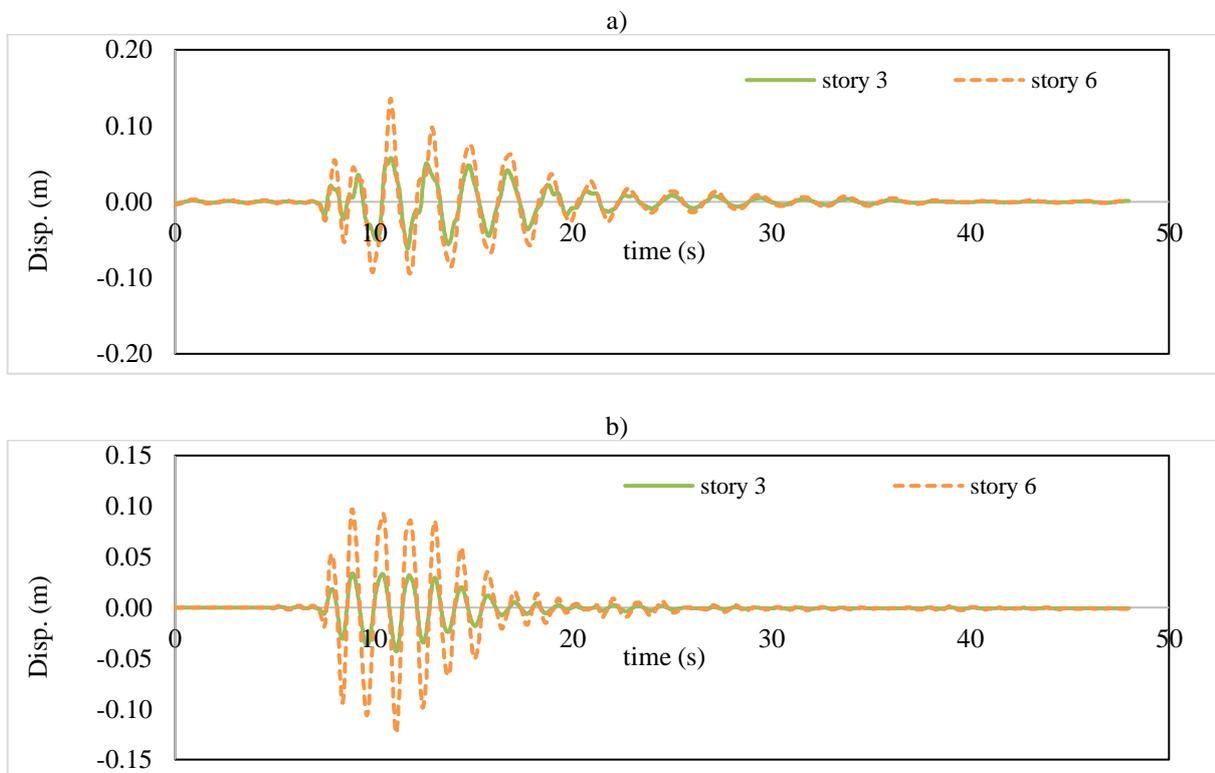
Fig. 6: The displacement of the 3<sup>rd</sup> and 6<sup>th</sup> story a) building with moment resisting frame system b) building with dual system
