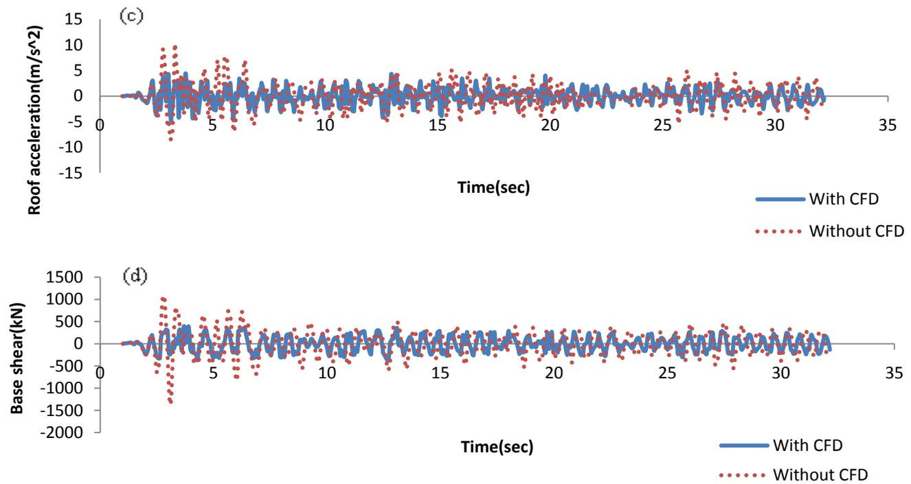
**Fig.9:** Response of the frame with and without damper: a) displacement of the roof, b) velocity of the roof, c) acceleration of the roof, d) Base shear.
