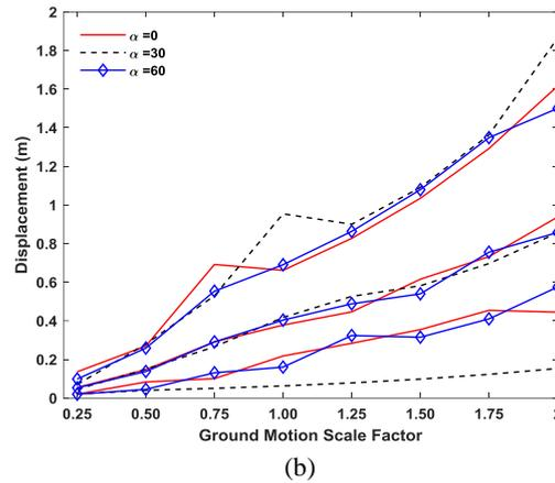
**Fig. 4:** Evolution of deck obtuse corner displacement with increasing intensity of GMs, including minimum, maximum and mean displacements (models F2S0, F2S30, F2S60), a) longitudinal direction, b) transverse direction
