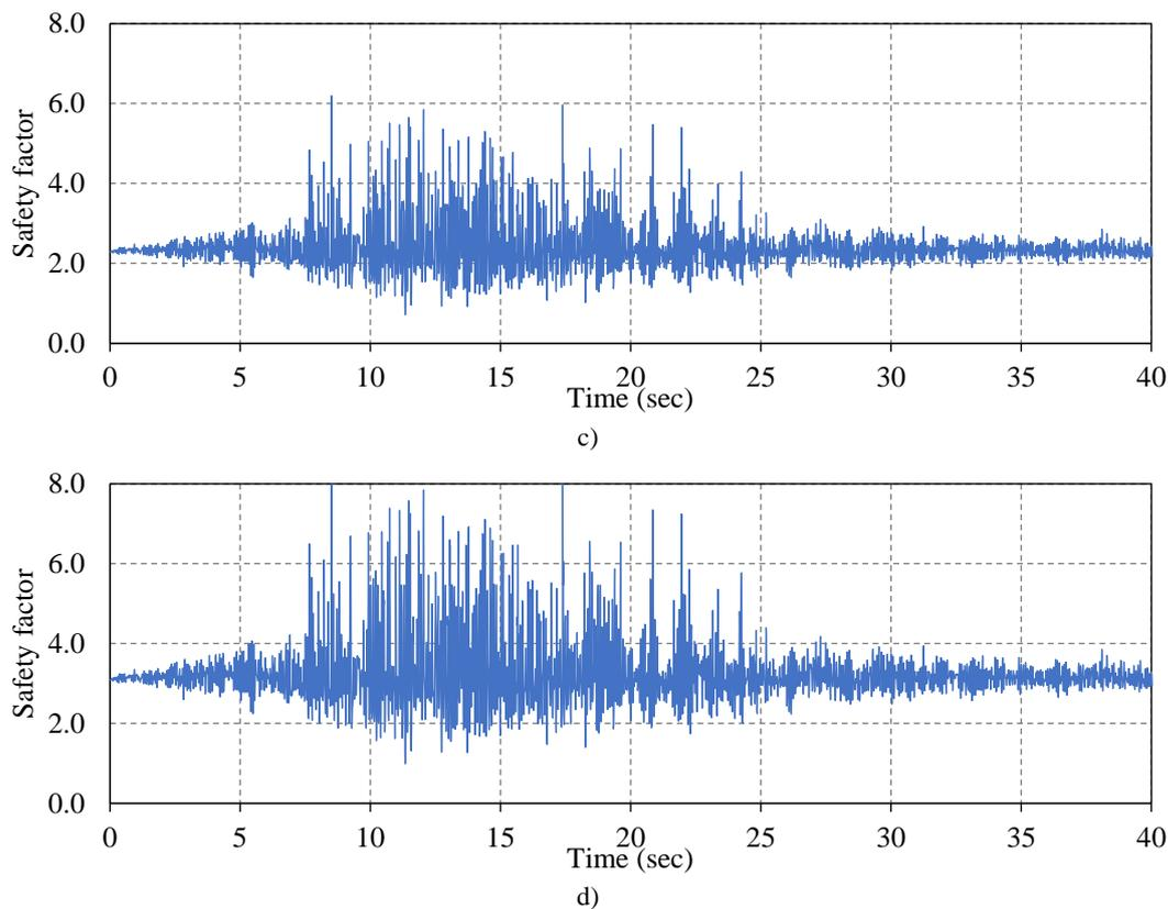
**Fig. 6:** The time histories of safety factors of WL6 wedge at the left abutment for different values of the friction coefficient. a)  $\mu = 0.25$  b)  $\mu = 0.50$  c)  $\mu = 0.75$  d)  $\mu = 1.00$
