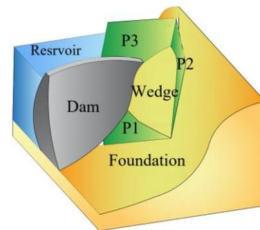
Fig. 1: Dam-reservoir-foundation, wedge, and its supporting planes.
