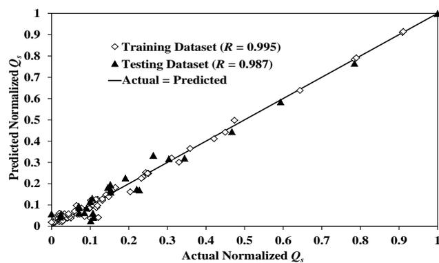
Fig.10: Performance of MARS model for drilled shafts.
