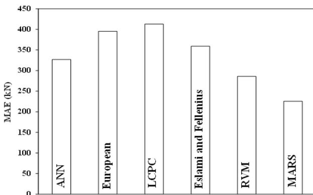
Fig.12: Bar charts of MAE for different models of driven piles.
