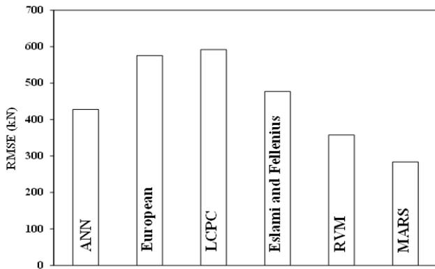
Fig.11: Bar charts of RMSE for different models of driven piles.
