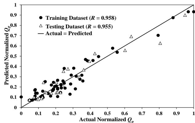
Fig.9: Performance of MARS model for driven piles.
