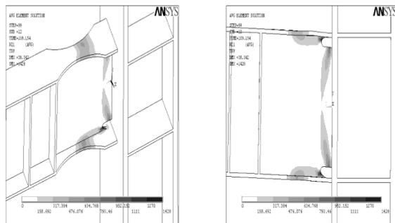
**Fig. 9:** Location of fracture in the intermediate link with reduced beam section and lateral bracing ( $\gamma_p = 0.02^{rad}$ )
