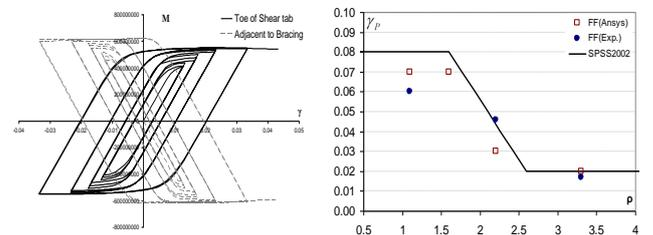
**Fig.7:** a) Hysteric loop at the end of shear tab and adjacent to bracing connection (long link)
