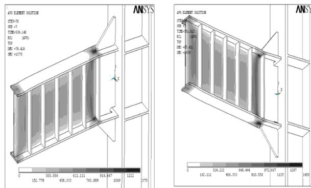
**Fig. 15:** Location of fracture in short link ( $e = 1.6M_p/V_p$ ) ( $\gamma_p = 0.08^{rad}$ )
