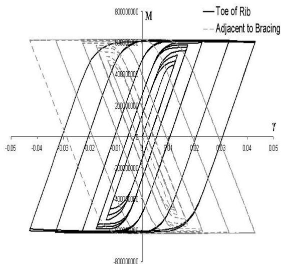
**Fig. 17:** a) Hysteric loop at the toe of Rib and adjacent to bracing connection (long link)
