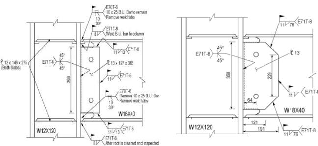
**Fig.4:** Connection details for short and long links
