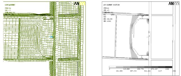
**Fig.6:** a. The shape of link deformed at the connection
