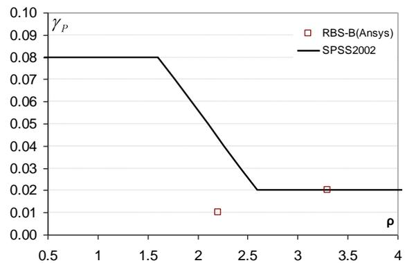
**Fig. 11:** comparing the analytical results and code provisions
