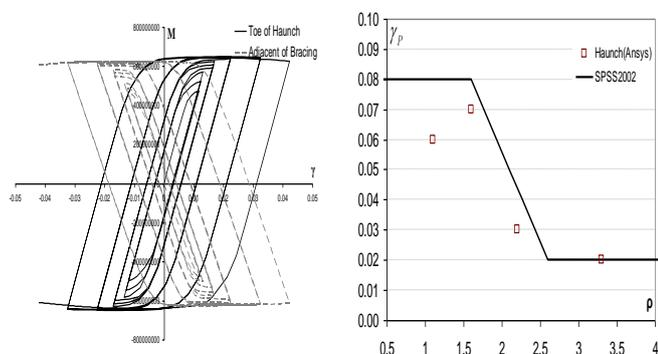
**Fig. 14:** a) Hysteric loop at the toe of haunch and adjacent to bracing connection (long link)
