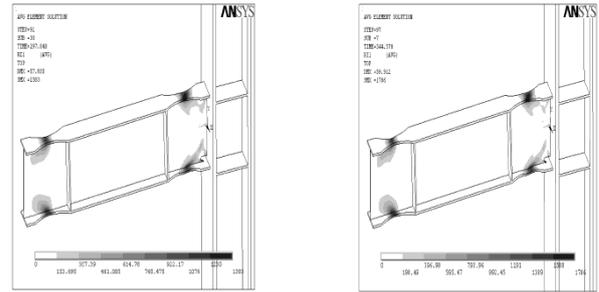
**Fig. 10:** Location of fracture in the intermediate link with reduced beam section and lateral bracing ( $\gamma_p = 0.03^{rad}$ )
