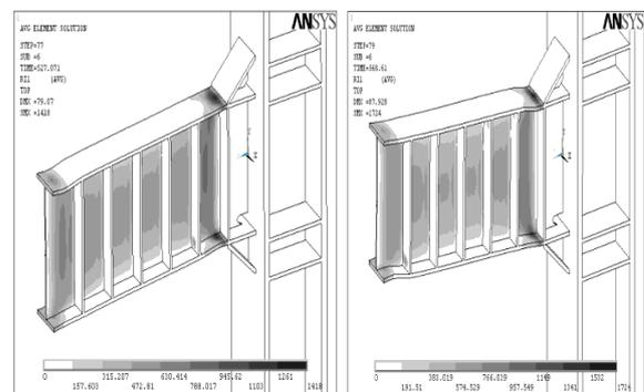
**Fig. 12:** Location of fracture in short link ( $e = 1.6M_p/V_p$ ) ( $\gamma_p = 0.08^{rad}$ )
