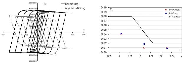
**Fig. 3:** a) Hysteric loop at column face and adjacent to bracing connection
