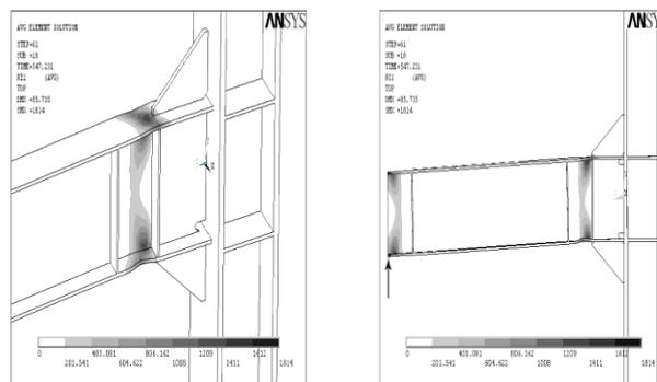
**Fig. 16:** Location of fracture in long link ( $\gamma_p = 0.03^{rad}$ )
