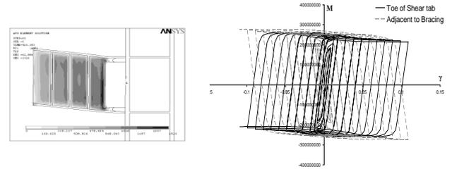
**Fig. 5:** a) Location of fracture in short link (at link the web, around the shear tab) ( $\gamma_p = 0.08^{rad}$ )
