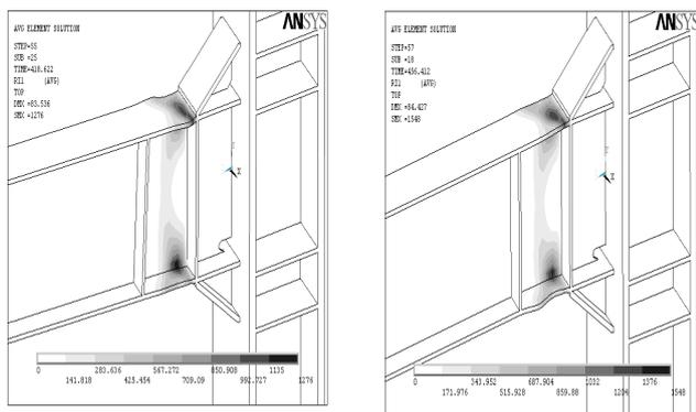
**Fig. 13:** Location of fracture in long link ( $\gamma_p = 0.03^{rad}$ )
