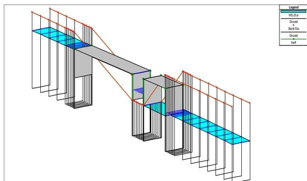
**Fig. 7:** Diagram of surface water profile at the junction with the bridge (discharge 25-year return period)
