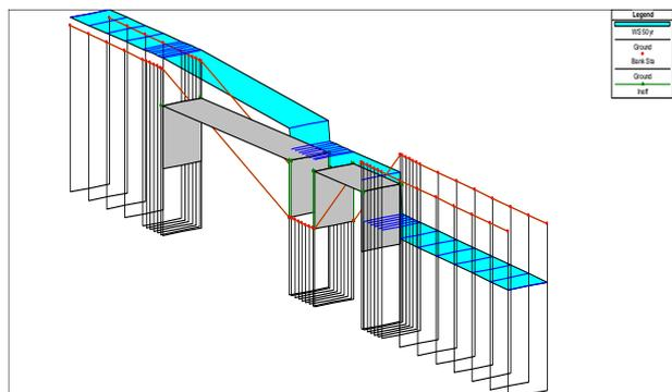
**Fig. 8:** Diagram of surface water profile at the junction with the bridge (discharge 50-year return period)
