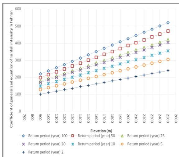
**Fig. 4:** Calculation chart of  $C_{Alt}$  coefficients using altitude (m) and return period (year) for Tehran
