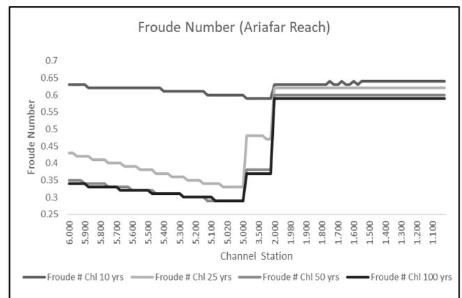
**Fig. 13:** Froude number profile obtained by hydraulic simulation for Mianroud canal (Ariafar Bridge)
