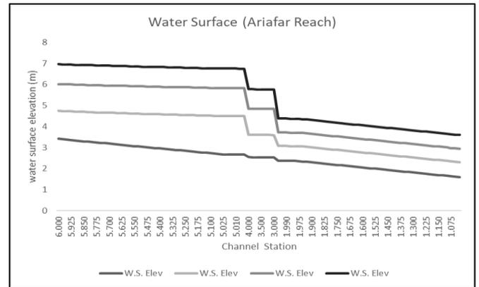
**Fig. 12:** Water surface profile obtained by hydraulic simulation for Mianroud canal (Ariafar Bridge)
