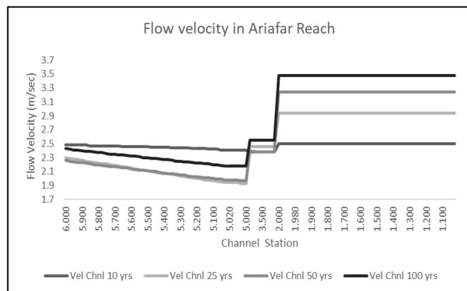
**Fig. 11:** Flow velocity obtained by hydraulic simulation for Mianroud canal (Ariafar Bridge)
