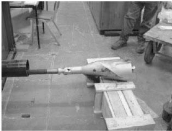
Fig.4: Clampburster pipe splitting device (from Rogers et al. 2002)
