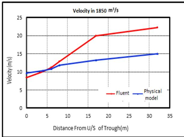
**Fig. 9:** A comparison of the numerical velocity results to the physical model data at 1850 m<sup>3</sup>/s
