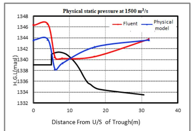
**Fig. 12:** A comparison of the numerical and physical static pressure results at 1500 m<sup>3</sup>/s
