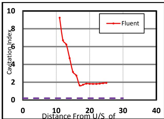
Fig. 14: A comparison of the cavitation index results at 35 m<sup>3</sup>/s
