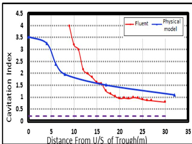
Fig. 15: A comparison of the numerical and observation cavitation index results at 800 m<sup>3</sup>/s
