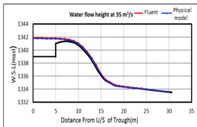
**Fig. 2:** A comparison of the numerical spillway water surface level profile and observation data at a flow rate of 35 m<sup>3</sup>/s
