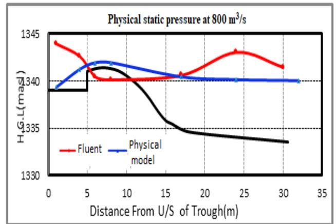
**Fig. 11:** A comparison of the numerical and physical static pressure results at 800 m<sup>3</sup>/s
