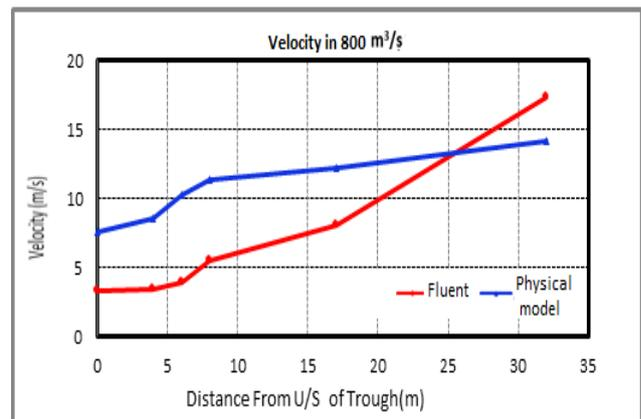
**Fig. 7:** Comparing the numerical velocity results to the physical data
