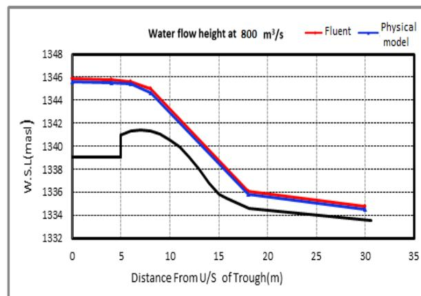
**Fig. 3:** A comparison of the numerical spillway water surface level profile and observation data at a flow rate of 800 m<sup>3</sup>/s
