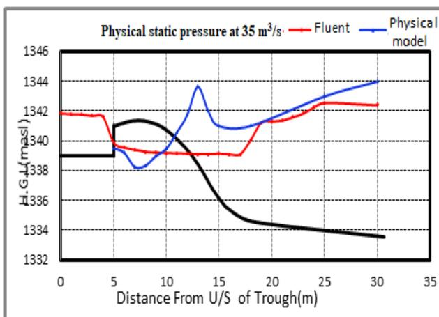
**Fig. 10:** A comparison of the numerical and physical static pressure results at 35 m<sup>3</sup>/s
