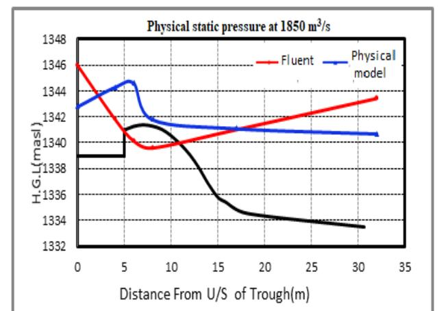
**Fig. 13:** A comparison of the numerical and physical static pressure results at 1850 m<sup>3</sup>/s
