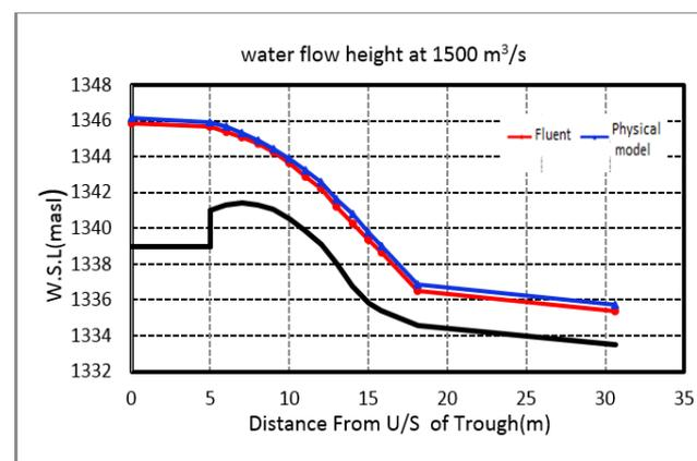
**Fig. 4:** A comparison of the numerical spillway water surface level profile and observation data at a flow rate of 1500 m<sup>3</sup>/s
