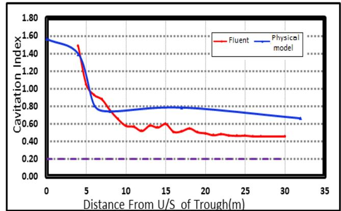
Fig. 16: A comparison of the numerical and observation cavitation index results at 1500 m<sup>3</sup>/s
