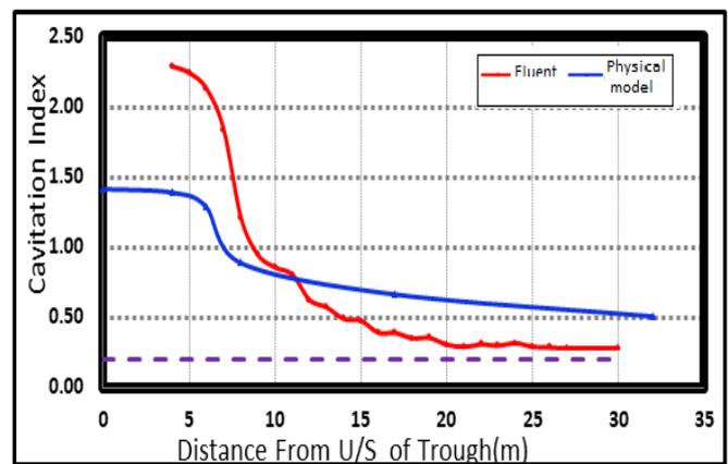
Fig. 17: A comparison of the numerical and observation cavitation index results at 1850 m<sup>3</sup>/s
