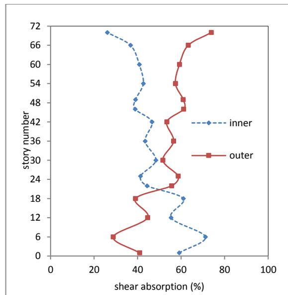
Fig. 30: Percentage of shear absorption of inner and outer tubes of T72TO-X.
