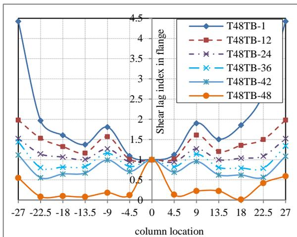
**Fig. 8:** The diagrams of shear lag index of flange in T48TB-SH (48-story building with tube in tube system and chevron-bracing on outer tube) at different stories
