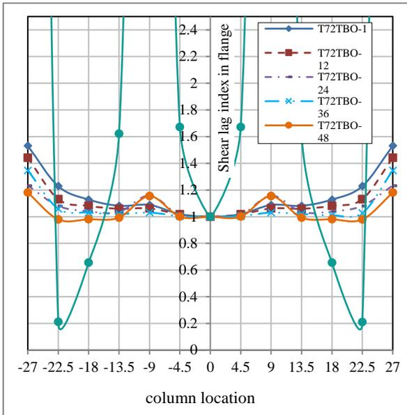
**Fig. 13:** The shear lag index of flange in T72TBO-X (72-story building with tube in tube system and X- belt trusses).
