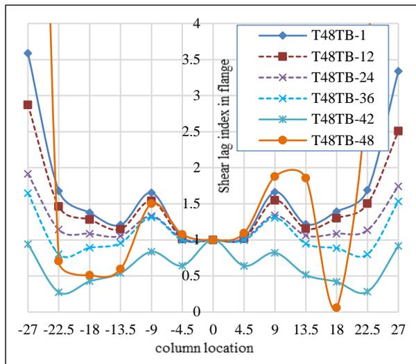
**Fig. 7:** The diagrams of shear lag index of flange in T48TB (48-story building with tube in tube system and X-bracing on outer tube) at different stories.
