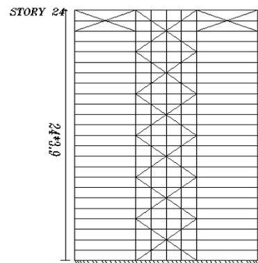
Fig. 2: A sample of X-belt truss the in the 24-story building.
