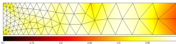
Fig.7: mesh quality for beam example in last step
