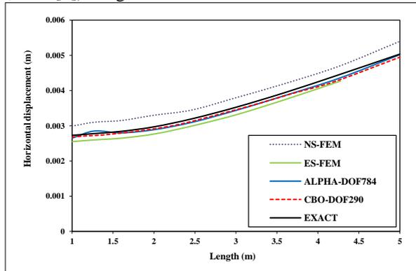
Fig.14: The horizontal displacement on the ED edge
