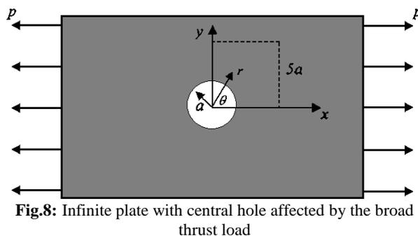
Fig.8: Infinite plate with central hole affected by the broad thrust load
