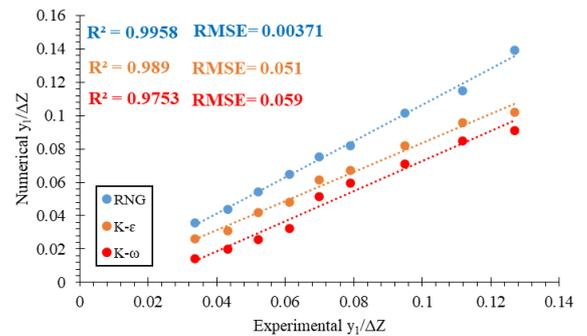
**Fig. 6:** Numerical and laboratory comparison of the downstream relative depth
