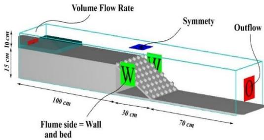
**Fig. 4:** Geometric profile of inclined drop and boundary conditions with the bat-shape roughness element
