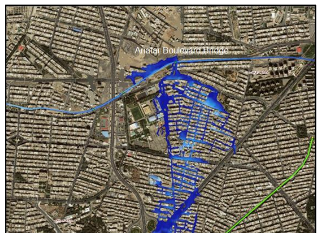
Fig. 10: 100-year flood zone map in the area of Ariafar Bridge
