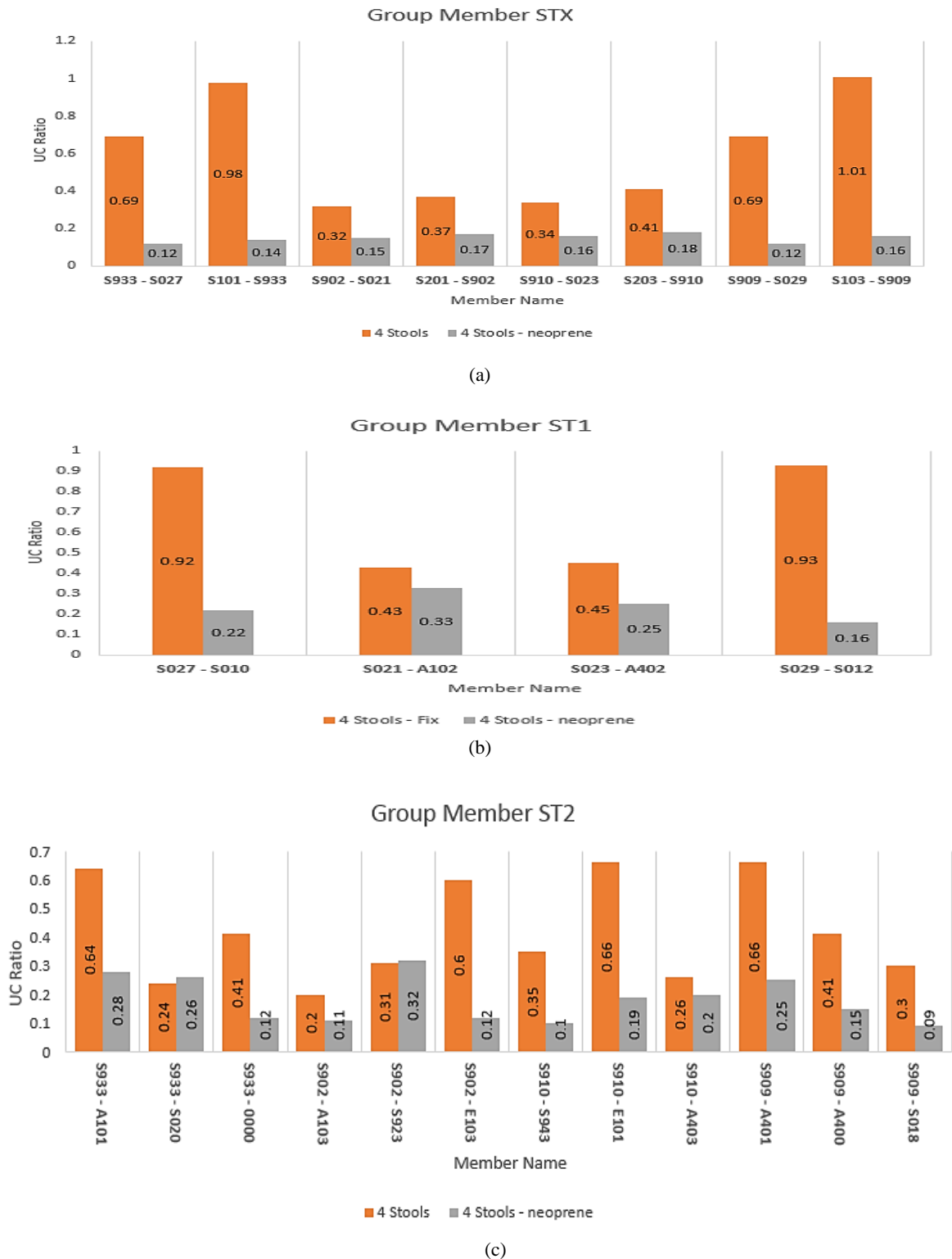
Fig. 11: Diagram of the Comparison between the members of the first area in the first a second model (a) STX group (b) ST1 group (c) ST2 group
