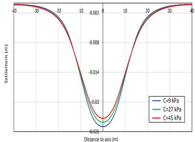
**Fig. 8:** Surface settlement curve for different Cohesions
