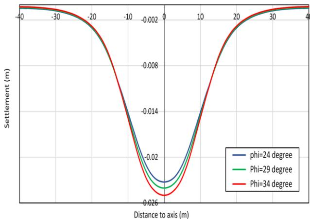
Fig. 9: Surface settlement curve for different friction angles
