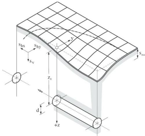
Fig. 1: Three-dimensional ground settlement due to tunnel excavation.
