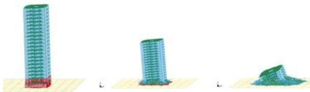
Fig.13: The process of a progressive collapse of the building.
