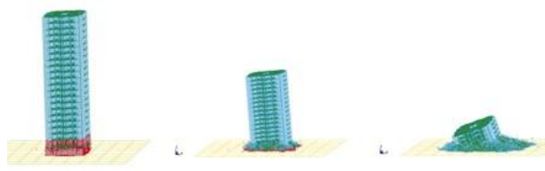
Fig.13: The process of a progressive collapse of the building.
