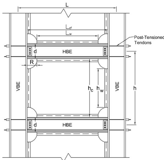
Fig. 1: Self-centering steel plate shear wall setup
