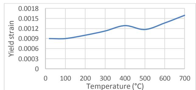
Fig. 14: Yield strain-temperature curve based on Eurocode 3 reduction factors
