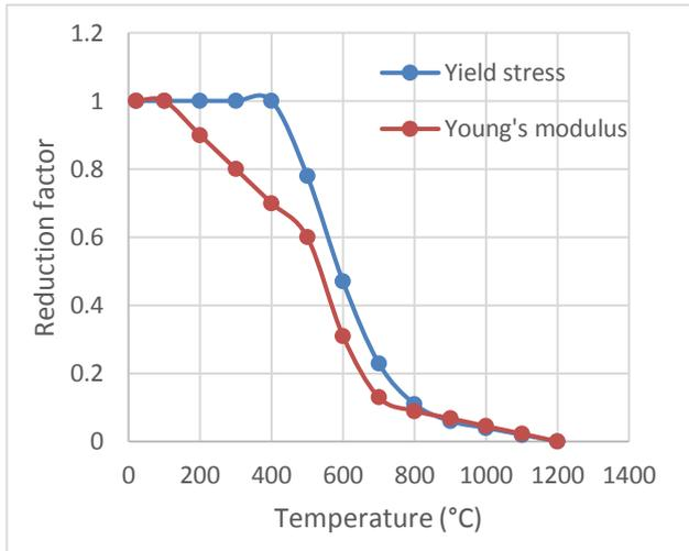
Fig. 9: Fire diagram in accordance with Eurocode 3 [19]
