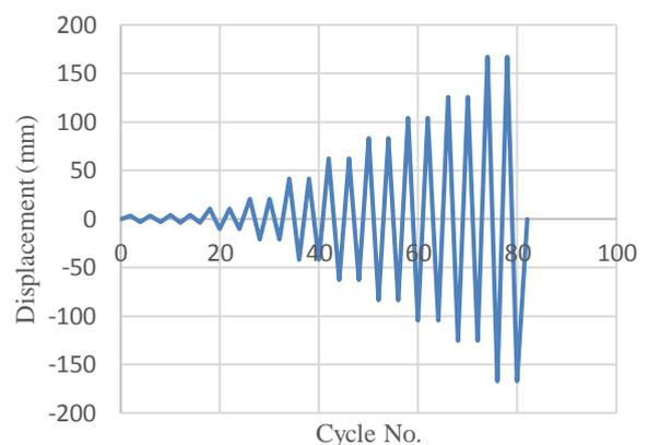
Fig. 6: The cyclic loading protocol for the SC-SPSW, based on ATC-24 [18]
