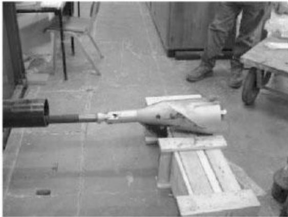
**Fig.4:** Clamburster pipe splitting device (from Rogers et al. 2002)
