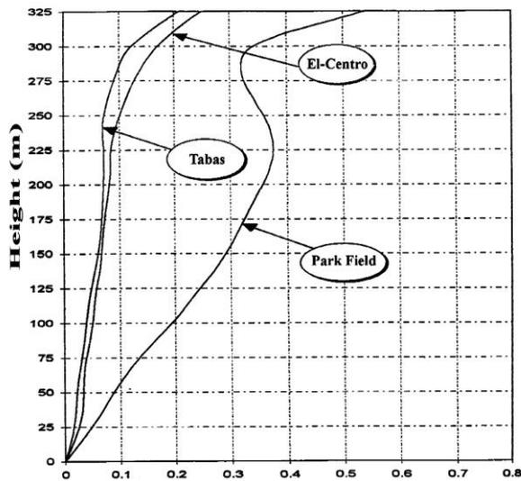
Fig 6-b: Max. displacement along tower (m), (0.25g)
