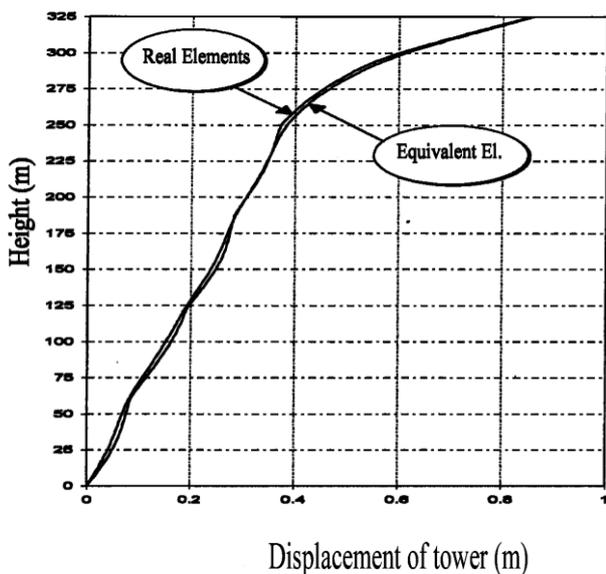
Fig.3: Typical comparison of model and structure deformation
