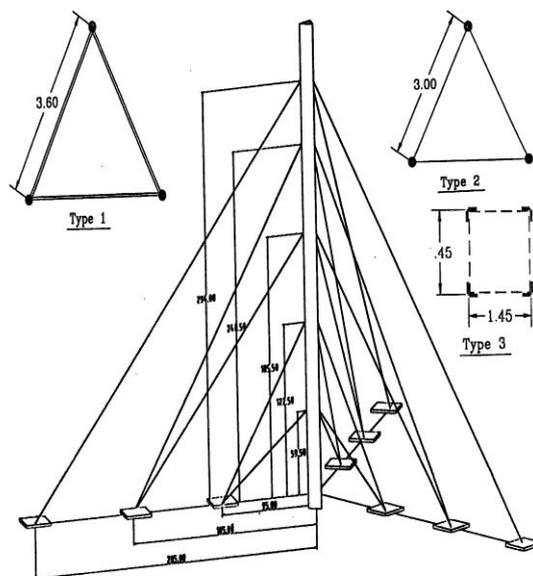
Fig. 4-a: Tower and space truss cross sections
